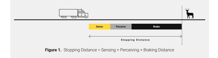
Under ideal circumstances, the road is straight and flat, the weather is dry and sunny, the driver is alert and law-abiding with a keen mind, the brakes are properly sized for the load with unworn pads, and the tires have good treads and proper air pressure. In this case, stopping distance is minimized and predictable based on vehicle speed and the coefficient of friction.
